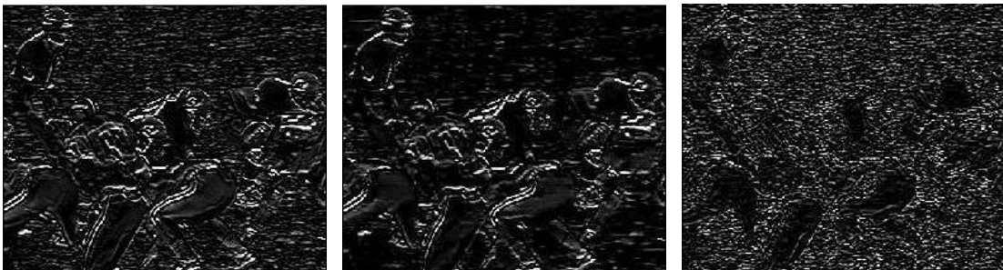
Figure 2.14 – Football SI (from left to right: original image filtered with Sobel edge filter, encode image filtered with Sobel edge filter, image difference)
