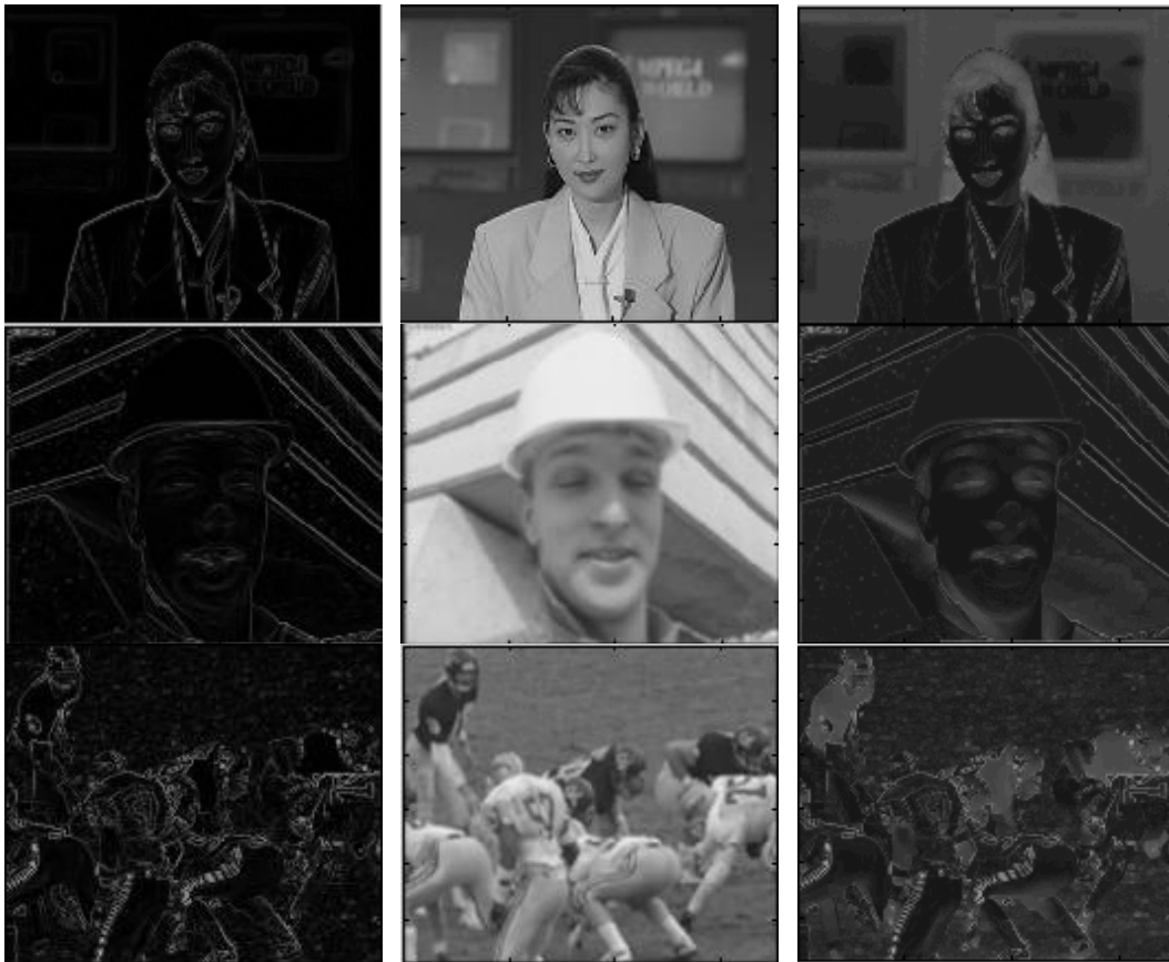
Figure 2.19 – JND Maps (from left to right: mg , bg and JND profile; from top to bottom: Akiyo sequence, Foreman sequence, Football sequence)
