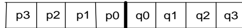
Figure 3.16 – Pixels on either side of a vertical boundary of adjacent blocks P and Q ([299])
