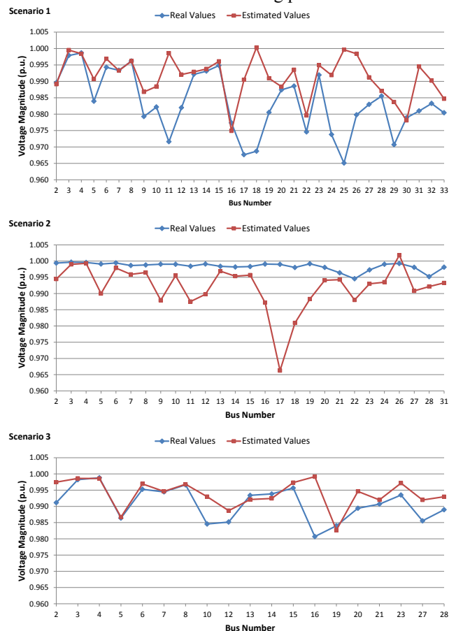
Fig. 7. Estimated and real values of voltage magnitude for the test sample with the highest absolute error in scenario 1, 2 and 3
