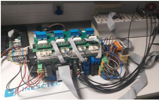
Fig. 13. PQ controlled active rectifier.
