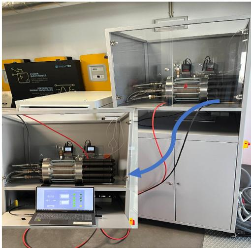
Fig. 14. 5kW PEM electrolyzer.
