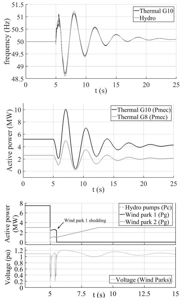
**Fig. 3** Windy valley scenario - Fault in the most loaded distribution feeder, plus the shedding of wind park 1 at 51 Hz
