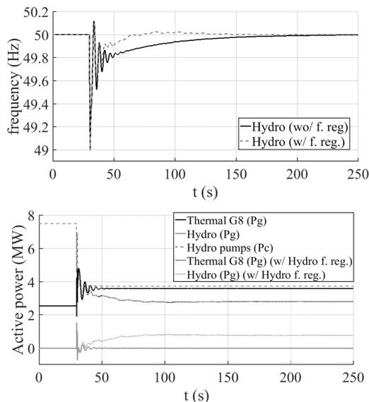
**Fig. 1** Windy valley scenario - G10 loss with/without freq. regulation provided by the hydro turbine, plus the shedding of 3 hydro pumps at 49 Hz. Legend: Pg and Pc – active power generation and consumption; f. reg – primary and secondary frequency regulation
