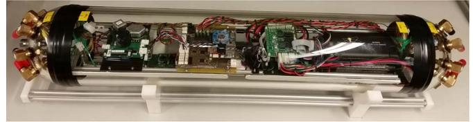
Fig. 5. Frame with onboard electronics installed inside the pressure housing.
