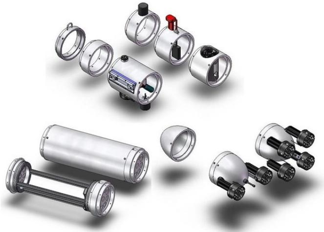
Fig. 1. Example of stackable AUV modules with 200m diameter. These include pressure housings, flooded extensions, and end sections.
