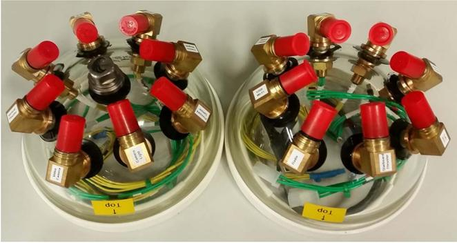
Fig. 3. DART pressure housing end caps, with right angle bulkheads installed in glass hemispheres. The bow end cap in the right-hand side has a vent port in the center.
