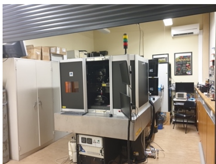
Main fabrication set-up for femtosecond laser writing at three wavelengths (342, 515 and 1030nm). The system uses translation and galvanometric scanning, together or independently.
