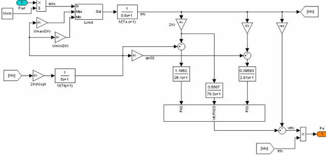
Fig. 10. SOFC model for the *Matlab® Simulink®* simulation platform
