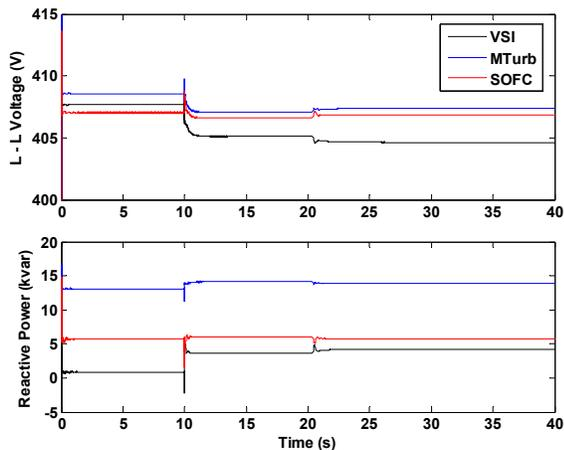
Fig. 14. Microsources voltages (rms values) and reactive powers
