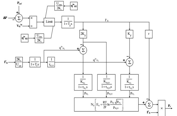
Fig. 2. SOFC block diagram model
