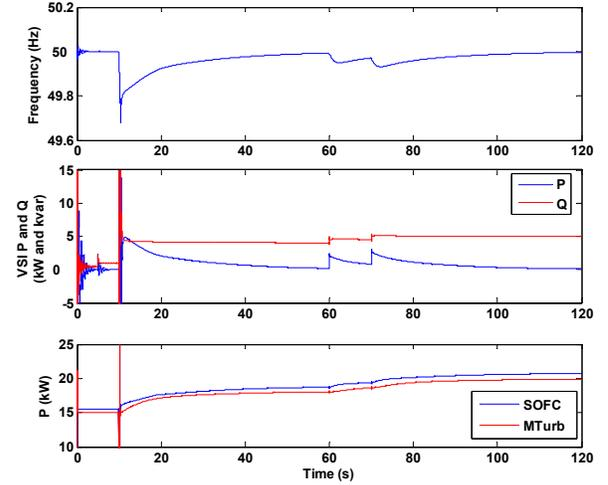
Fig. 11. MG Frequency, VSI active and reactive power and SOFC and single-shaft microturbine active power
