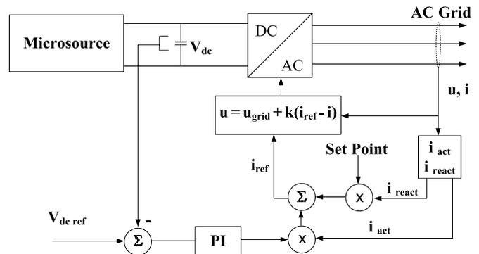
Fig. 3. PQ inverter control system
