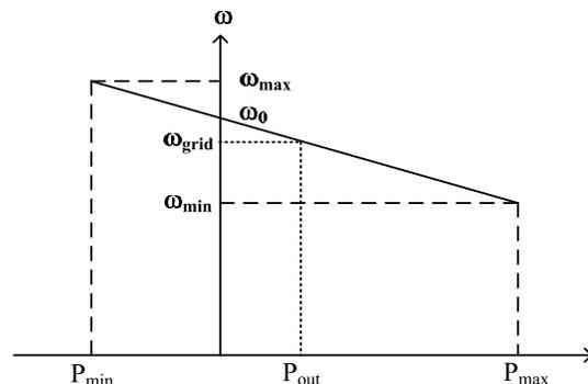
Fig. 4. Frequency / active power droop characteristic
