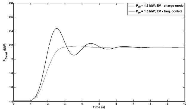
Fig. 7. Diesel units active power for scenario 1.
