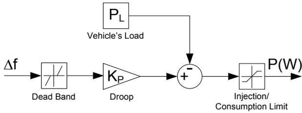
Fig. 4. Control loop for EVs active power set-point.
