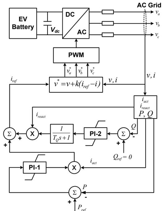
Fig. 3. PQ inverter control system [1].
