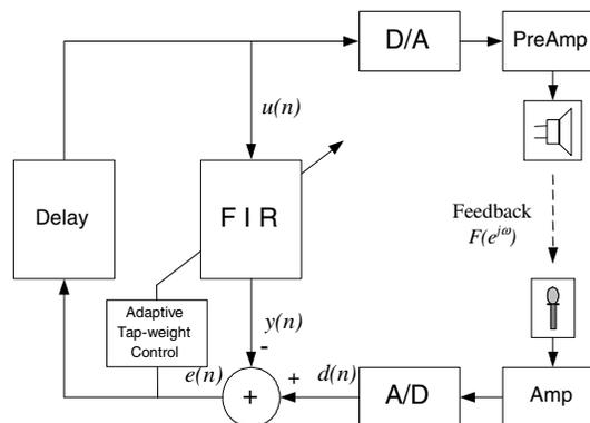
Figure 2: Adaptive FIR filtering applied to cancel acoustic feedback.
