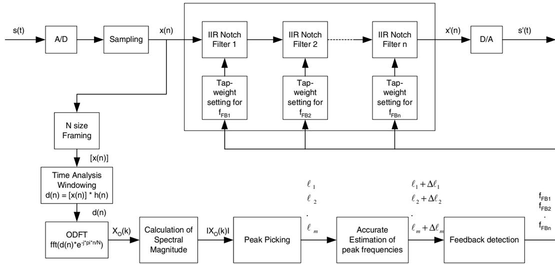
Figure 8: General Algorithm of the Multiple Feedbacks Canceller.
