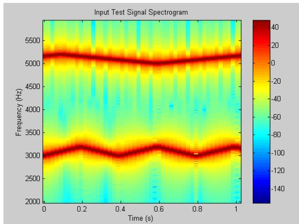
Figure 10: Input signal spectrogram for two simultaneous variable frequency test sinusoids.
