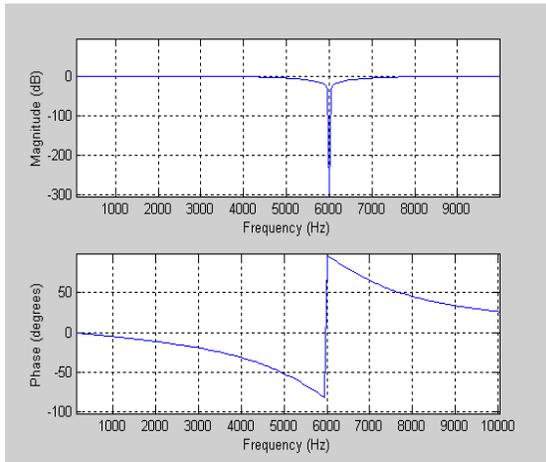
Figure 6: Notch Filter frequency response, including Magnitude (above) and Phase (below) curves.
