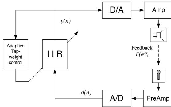
Figure 4: Adaptive IIR filtering applied to cancel acoustic feedback.
