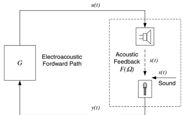
Figure 1: Schematic of an audio amplification system producing acoustic feedback.
