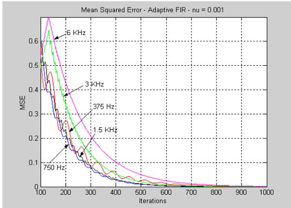
Figure 3: Learning Curves of the Adaptive FIR filter implemented on DSP, with  $\mu = 0.001$ , for different test frequencies.
