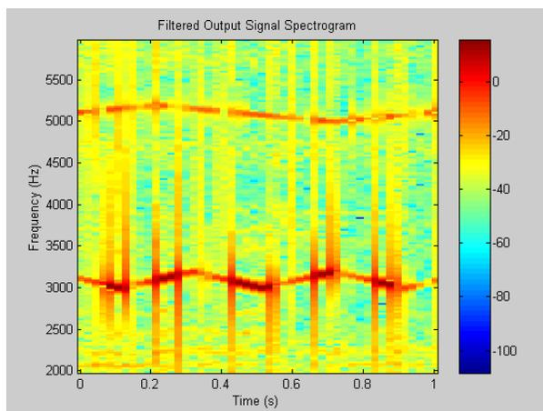
Figure 11: Output filtered signal spectrogram for two simultaneous variable frequency test sinusoids.
