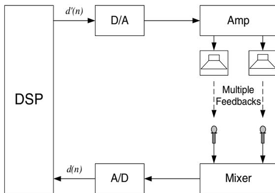
Figure 14: Double Acoustic Feedback generated by means two simultaneous couplings.
