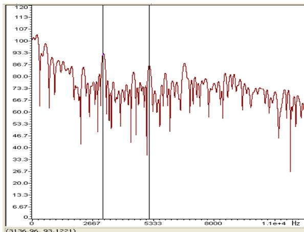
Figure 13: Filtered Output Signal Spectrum for two simultaneous variable frequency test sinusoids.
