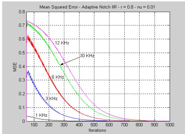
Figure 7: Adaptive IIR filter learning curves for different frequencies, with  $\mu = 0.01$  and  $r = 0.8$ .
