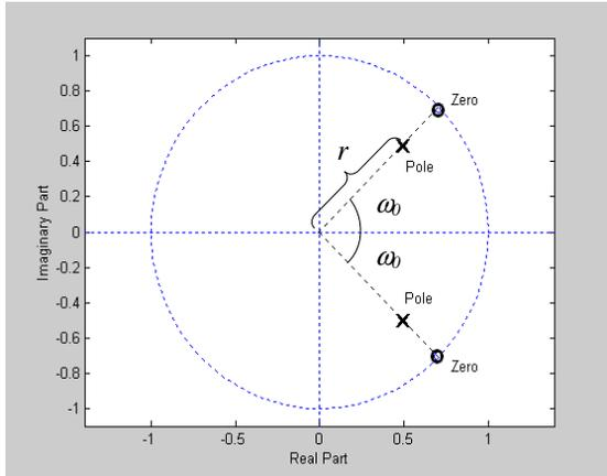
Figure 5: Zero-pole pattern of the Notch Filter Transfer Function
