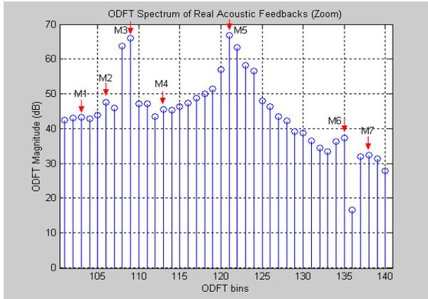
Figure 9: Partial view of the ODFT spectrum corresponding to an audio signal containing feedbacks. Local maxima are signaled.
