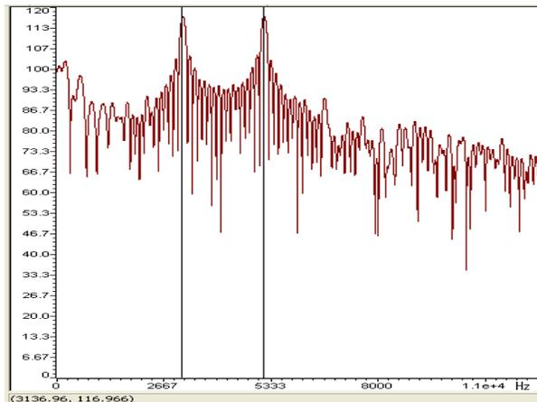
Figure 12: Input Signal Spectrum with two simultaneous variable frequency test sinusoids.
