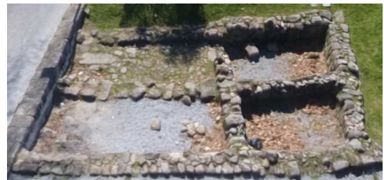
Fig. 4. Example of a Pix4D output as a result of photogrammetric processing upon imagery set regarding city gate's old ruin, situated in Vila Real (Portugal). Imagery was collected using a Phantom 4 flying at 40m of altitude, in double grid mode, with an overlap of 90% and 80° of camera orientation. 107 photos were taken in 4min and 10s. Some shadows burned in the 3D model reflect the influence of the light conditions (sunny day) over pictures acquisition task.
