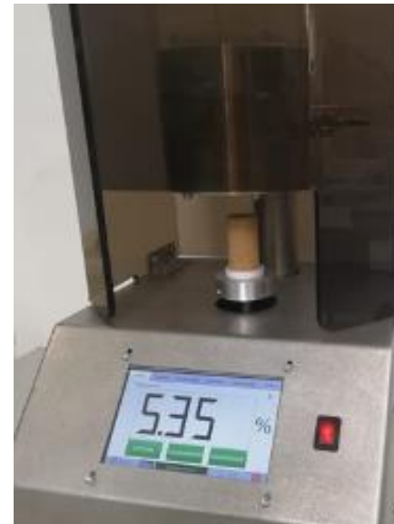
Microwave cavity for cork moisture measurement
