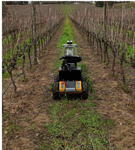
**Figure 4.** The AgRob V16 robotic platform recording data in one of the vineyards that compose the VineSet.
