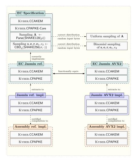
**Figure 1:** Overview of the proof structure and tooling. Elements in dashed boxes are automatically generated; elements in solid boxes need to be written by hand.
