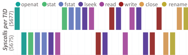
Fig. 3: Syscalls issued over time by RANSOMEXX's encryption threads to file F10573.bqt.vmdk.
