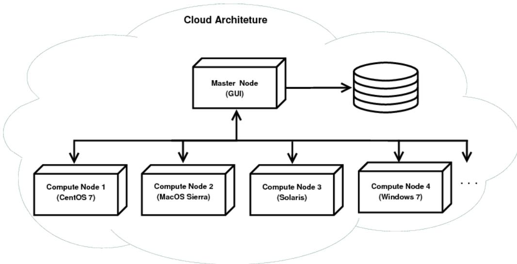
■ **Figure 3** The cloud-based architecture of YAPTBE
