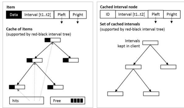
Figure 1: Dual red-black augment interval tree structure for cache of items (left) and cache of intervals (right).
