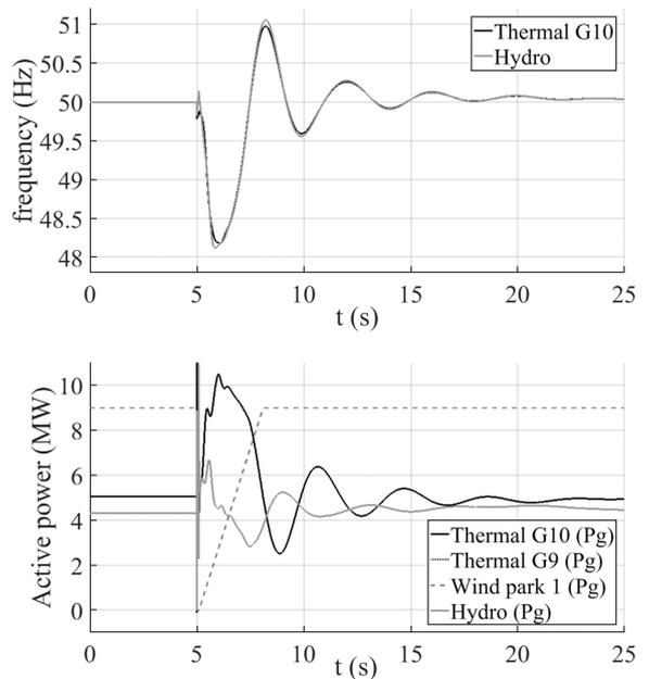
**Fig. 6** Maximum RES scenario - Fault in a transmission line, including an increased maximum active power recovery gradient in wind generators after a FRT situation
