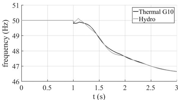
**Fig. 5** Maximum RES scenario - Fault in a transmission line
