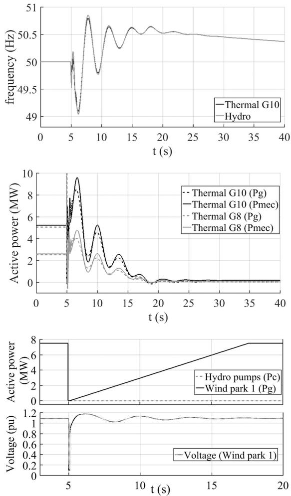
**Fig. 2** Windy valley scenario - Fault in a transmission line. Legend: Pmec - mechanical power
