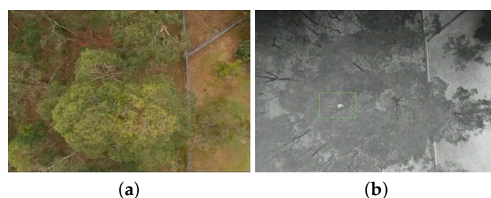
Figure 3. (a) RGB and (b) thermal images of a koala in its natural habitat captured at 60 m by a UAV, described in detail in [20].
