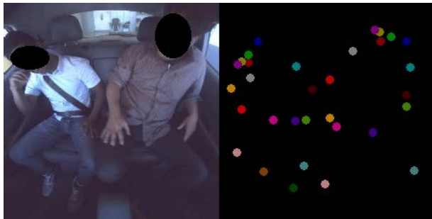
FIGURE 4. Key points calculated by the pose estimation model (Sunnyvale dataset from Bosch Car Multimedia).
