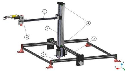
**Figure 5** Apple tree pruning manipulator rotary segment (Zahid *et al.*, 2020)
