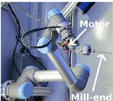
**Figure 3** Pruning manipulator on a mobile base
