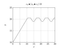
Clearly,  $c_3$  can be regarded as a supervisor system that, for the sake of efficiency, only acts when temperatures exceed the threshold, using just enough power to keep the temperature below the limit. Actually, note that  $c_3$  is able to play a supervisory role precisely because it is not pre-dynamical.
