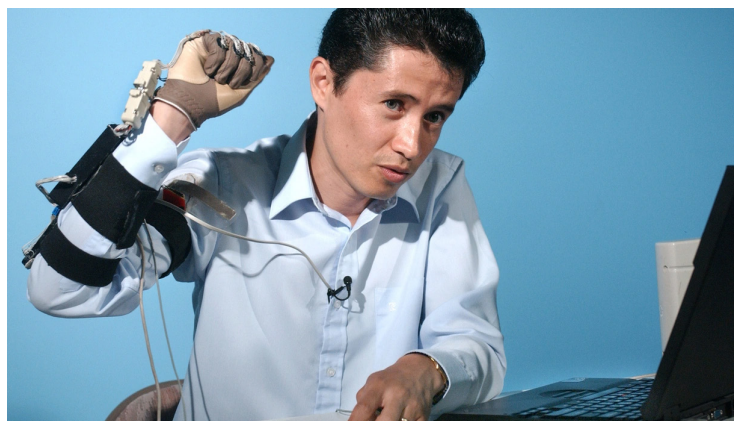
Figure 8: Prototype sign language sensor gloves (Erard 2017)
