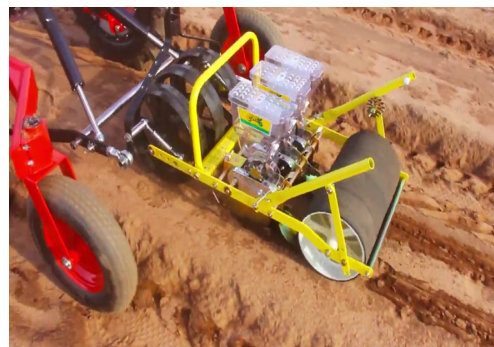
Figure 5. Di-Wheel's seeding mechanism [29].
