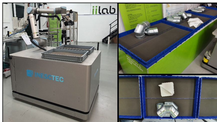
Figure 1. Use-case scenario: (Left) omnidirectional robot manipulator, (Right) bins.
