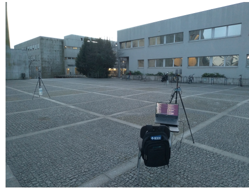
(b) Receiver placed along one of the edges of the outlined space, with laptop arrangement to store received BLE packet phase data from all four transmitters.
