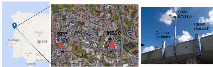
Fig. 2. Geographical setting: location map (left), location of the site and local meteorological station (middle) and measurement site (right).
