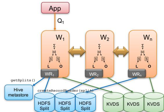
Figure 5. Parallel join between LeanXcale and HDFS tables.
